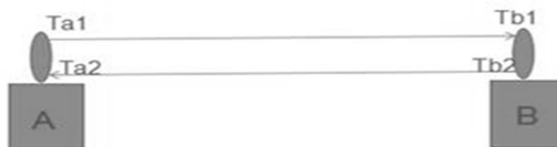
Fig. 1. Principle of UWB ranging
